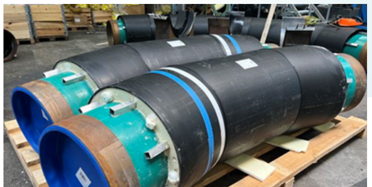
Hot Induction Bends insulated in Austria
