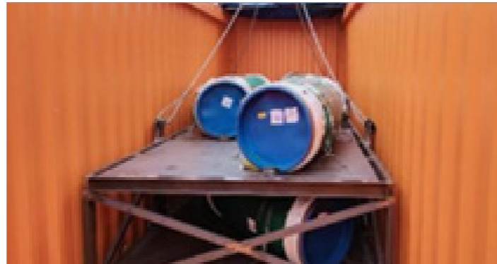
Bends packed and containerized
