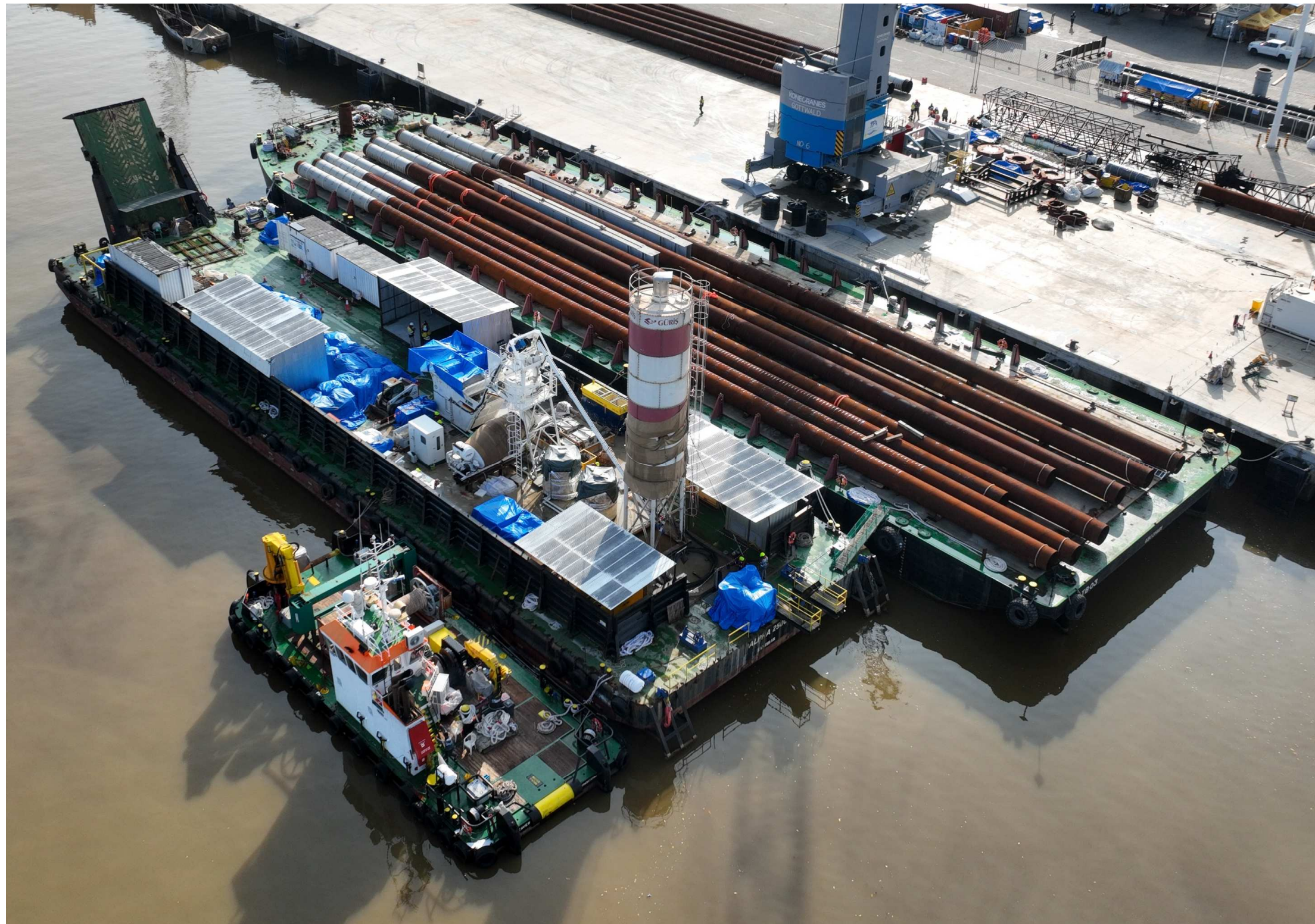
Finalizing the Trial Mix, Thermal Mock-up & Concrete Cube Test with our Floating Batching Plant.
