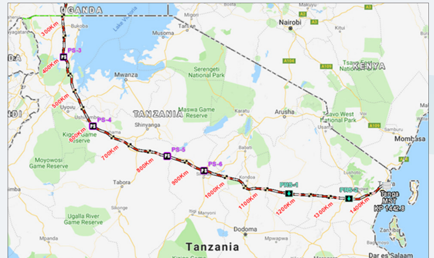
Location of EACOP pipeline route and permanent Above Ground Installations (AGIs) (PS: Pumping Stations, PRS: Pressure Reduction Stations, MST: Marine Storage Terminal)
