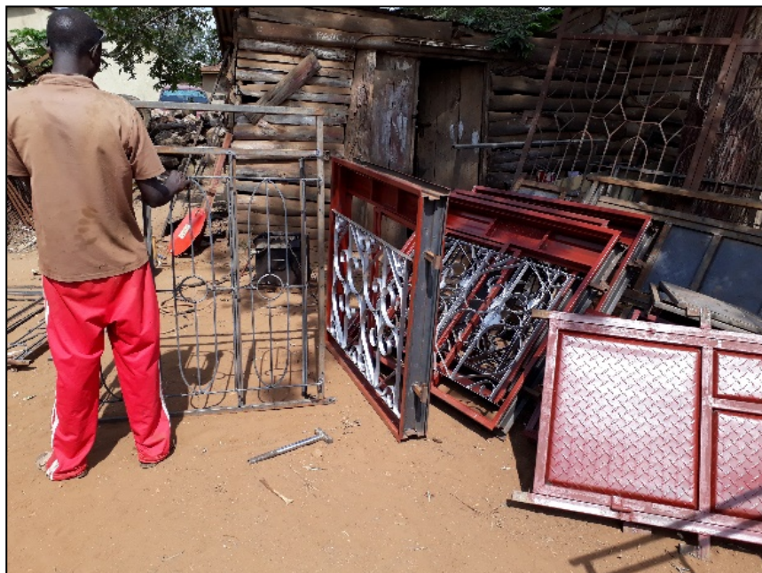
Figure 6-11: Steel work yard of artisan (fundu) manufacturing mild steel frame windows and burglar bars
