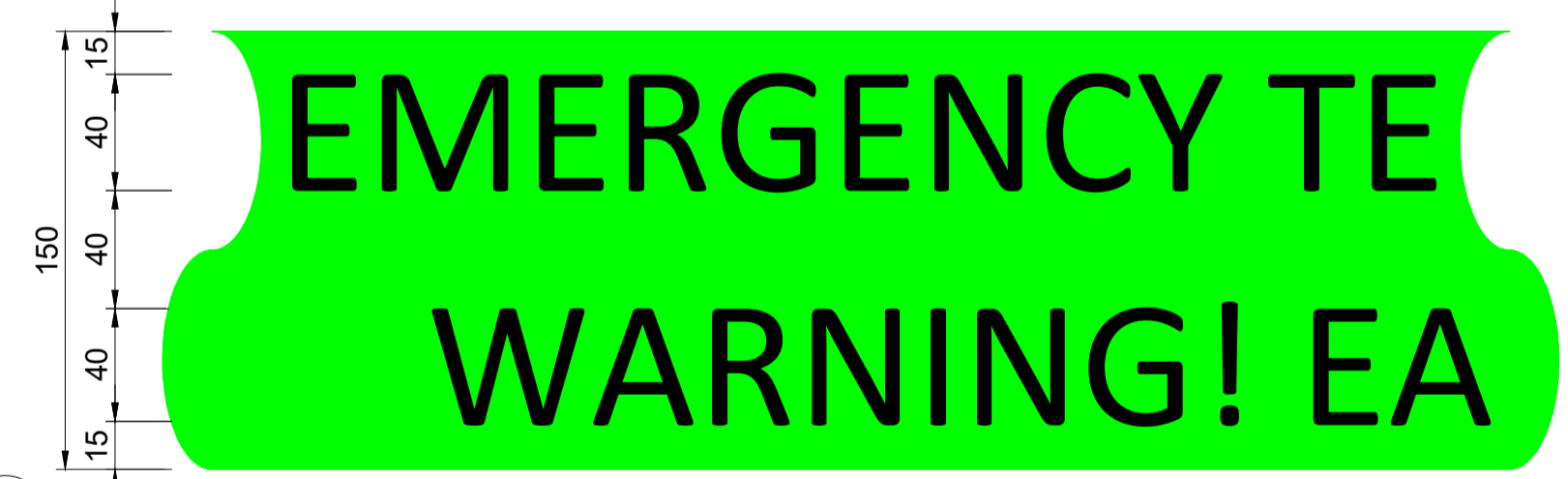
DETAIL 2 CABLE WARNING TAPE DIMENSIONS
