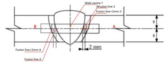
4) Test specimens shall be cut mechanically (sawing, milling). Flame cutting shall only be permitted to facilitate machining, and only if cuts are spaced at least 50 mm from any test specimens.
