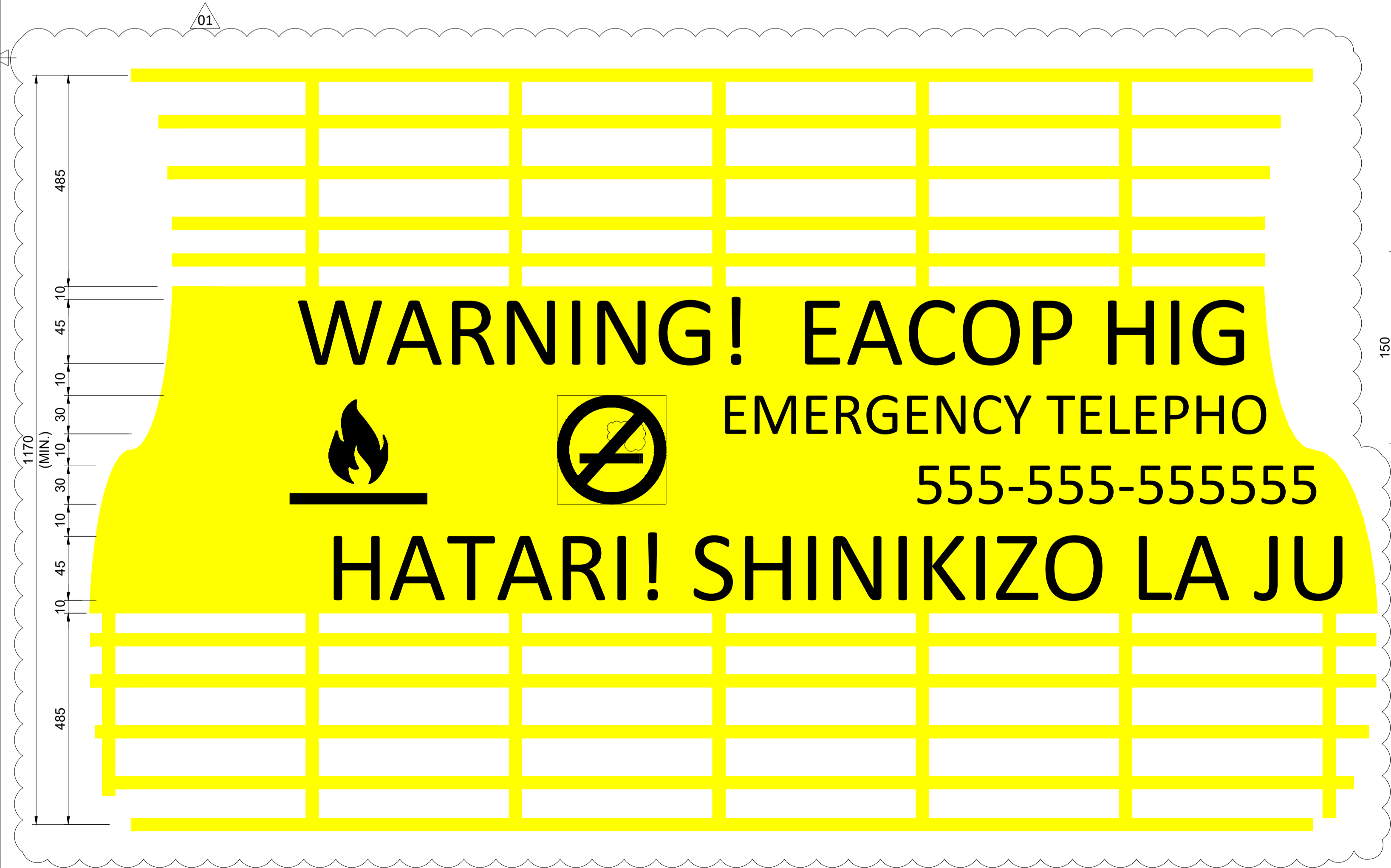
DETAIL 1 PIPELINE WARNING TAPE DIMENSIONS
